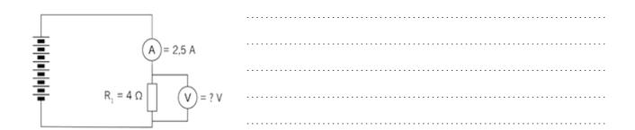
4. Calculate the resistance value of the resistor.
